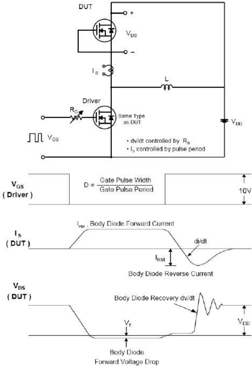
Fig 15. Peak Diode Recovery  $dv/dt$  Test Circuit & Waveforms
